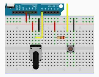
Connect center pin to A0, outer pins to (+) and (-) rails
