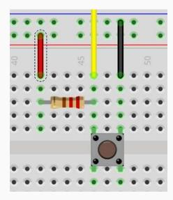
Reading a floating pin is **bad**. A switch only connects and disconnects a wire. When the wire is disconnected... the INPUT pin is floating!
