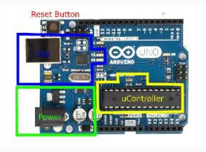
It's a kit (on a board) with the bare minimum components to easily use the  $\mu$ C hardware. They do the basic, boring design needed for any board, so users only need to add the neat stuff.
