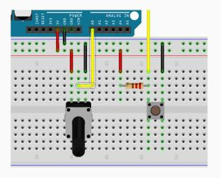
Connect center pin to A0, outer pins to (+) and (-) rails
