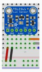
Connect Vin to (+) rail, GND to (-) rail, SDA to Arduino pin A4 and SCL to A5  $\,$
