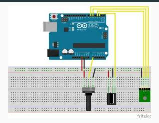
OUT of IR Receiver connects to pin 2 of Arduino, GND (middle) GND rail, remaining pin to Vcc rail.
